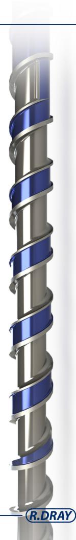
Melting area is only one ingredient in a successful screw design. Improper feeding and metering section designs can detract from a properly designed barrier section.
